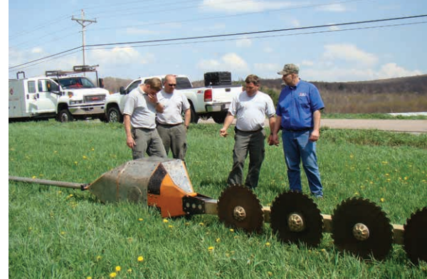
HELICOPTER WORK: Doug Glessner, the cooperative’s recently retired operations manager, discusses aerial right-of-way trimming with helicopter operators. This method of cutting is used in difficult to reach, cross-country terrain.
